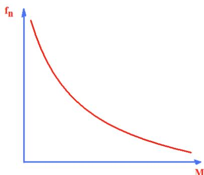
**Graph 1:** The relationship between the square of the resonant frequencies and mass density (linear density) when all other variables are held constant is an inverse curve. (That is:  $f_n \propto 1/\sqrt{M}$ )
