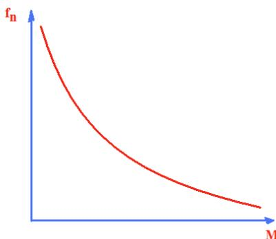
**Graph 3:** If the tension and length are fixed, and  $M$  is varied, the square of the resonant frequency will be inversely proportional to the square root of the mass of the string.
