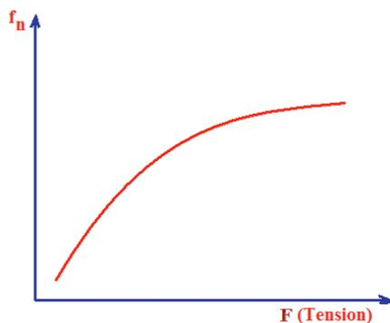
**Graph 3:** For a fixed length  $L$ , the resonant frequencies will be directly proportional to the square root of the tension in the spring. That is, functions produce the best fits through the points  $f_n \propto \sqrt{F}$
