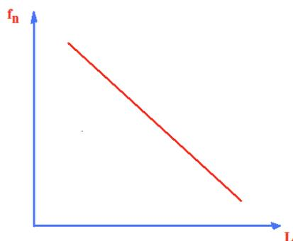
**Graph 2:** The relationship between resonant frequencies and the length of the spring when all other variables are held constant is an inverse curve. That is, functions produce the best fits through the points is:  $f_n \propto 1/L$
