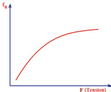
**Graph 1:** For a fixed length, the resonant frequency will be directly proportional to the square root of the tension in the string. The resultant is a curved graph.
