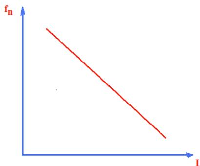
**Graph 2:** If the tension and linear density are fixed, the resonant frequency will be inversely proportional to the length of the string. In this case only the length is varied.
